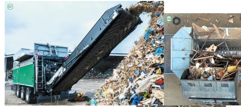
The highest possible shredding force is required for these inhomogeneous waste streams. The Terminator's powerful drive delivers it. The F or XXF units are used for these applications, depending on the desired degree of shredding.
